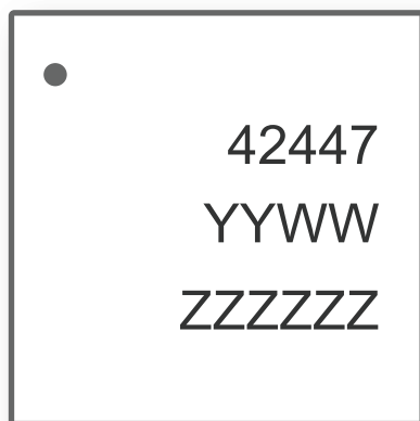
Figure 16 • Package marking specification
