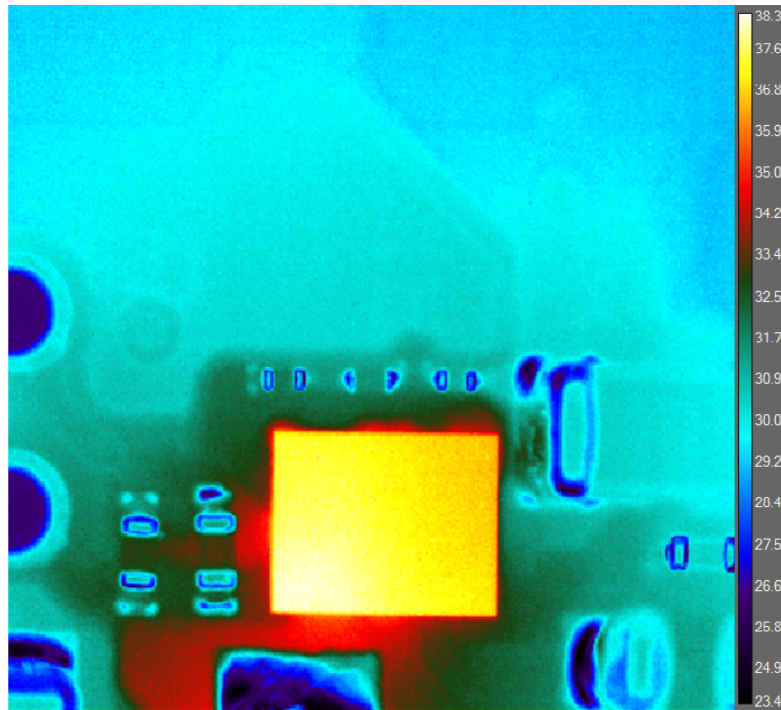
Figure 15. ARC1C0608 Thermal Performance 6p6s configuration, V_{OUT}=17.5V , 150 mA, V_{IN}=3V , 0.3W power dissipation, 1.2 mm 6.8 \mu H inductor (DFE322512F-6R8M, ambient temperature 24 °C Maximum temperature is 38.3 °C close to the LX and PGND pins of the package
