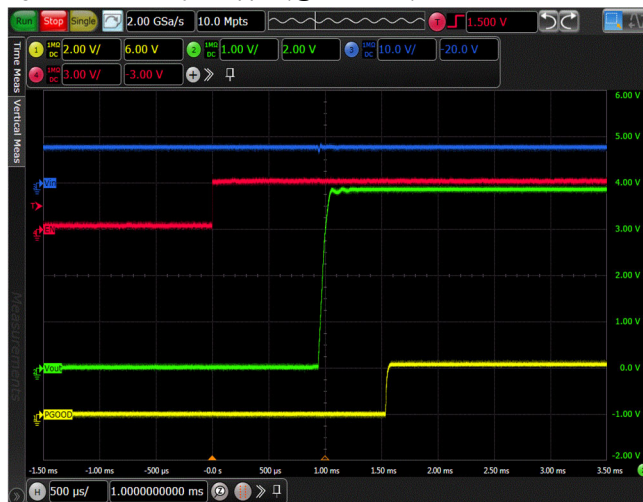
Figure 22. DIV2 Start up, C_{LOAD} = 100 \mu F
