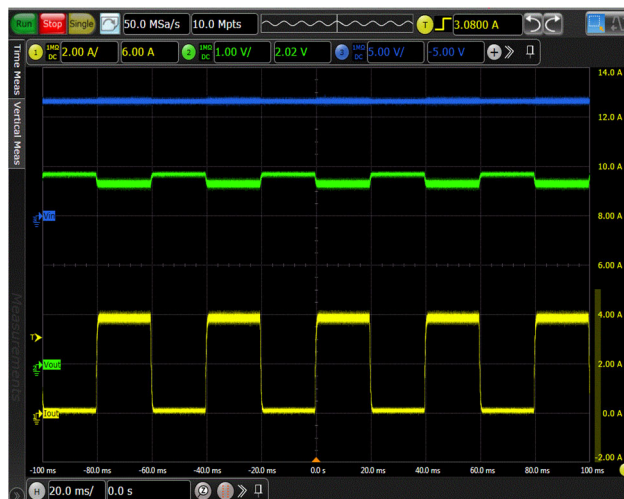
Figure 25. Load transient (0.1A - 4A) V_{IN} = 11.55V DIV3 C_{LOAD} = 100 \mu F
