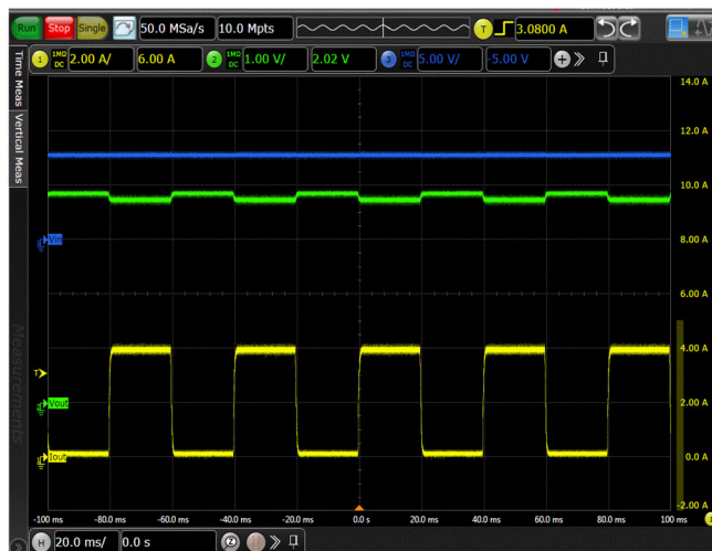
Figure 24. Load transient (0.1A - 4A) V_{IN} = 7.7V DIV2 C_{LOAD} = 100 \mu F
