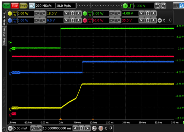
Figure 13. Startup behavior with V_{OUT} loaded with 100\Omega , within the soft-start timeout, V_{IN}=48V
