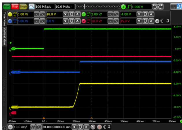
Figure 9. Power-up scope plot, no load, V_{IN}=48V , C_{LOAD} = 44\text{ }\mu F
