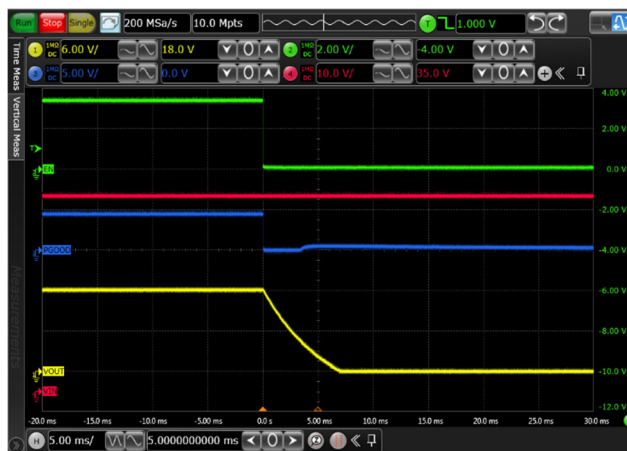
Figure 10. Shutdown behavior with V_{OUT} loaded, V_{IN}=48V , C_{LOAD} = 44\text{ }\mu F
