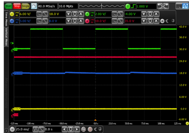
Figure 14. Startup into a short circuit, V_{IN} = 48V . The device latches off after a short circuit until EN is cycled.
