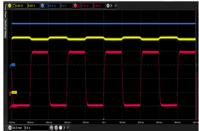
Figure 26. Load transient (0.1A - 8A) VIN=48V DIV 3 CLOAD = 80 \mu F, single operation
