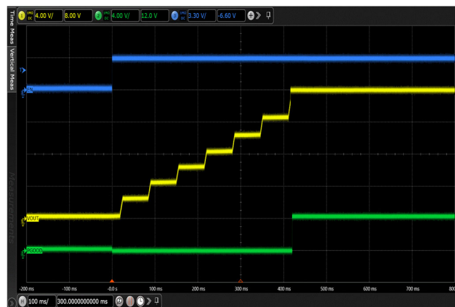
Figure 24. DIV 3 VIN = 48V start up, CLOAD = 80 \mu F, single operation
