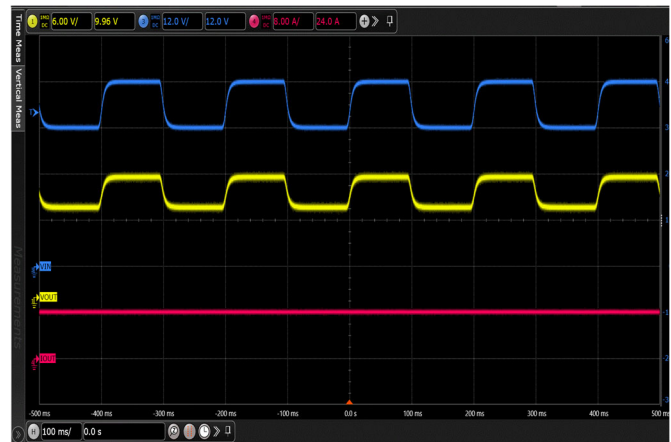
Figure 28. Line transient 36-48V ILOAD = 8A DIV 3 CLOAD = 80 \mu F single operation
