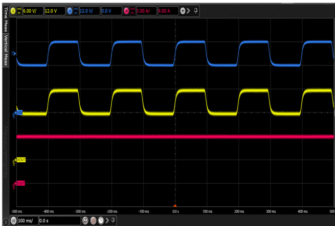
Figure 27. Line transient 24-36V ILOAD = 6A DIV 2 CLOAD = 80 \mu F single operation
