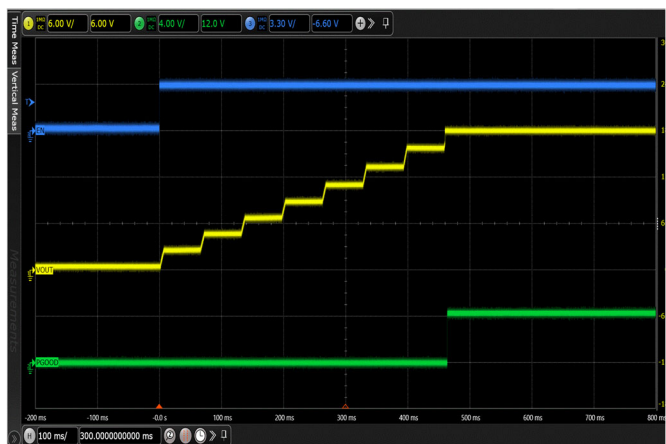
Figure 23. DIV 2 VIN = 36V start up, CLOAD = 80 \mu F, single operation
