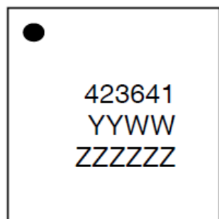
Figure 14. PE423641 package marking specification
