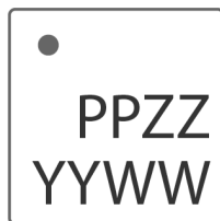
Figure 15. PE42429 package marking specification
