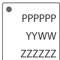
Figure 15. PE42544 package marking specification
