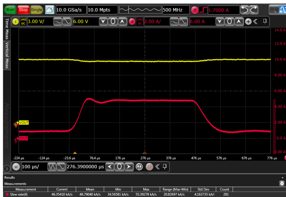
Figure 11. Load Transient Response ( V_{IN}=48V , 1 – 5A Load Step, 50A/ms) with Added 44\ \mu F Output Capacitance through 2\times 22\ \mu F Capacitors
